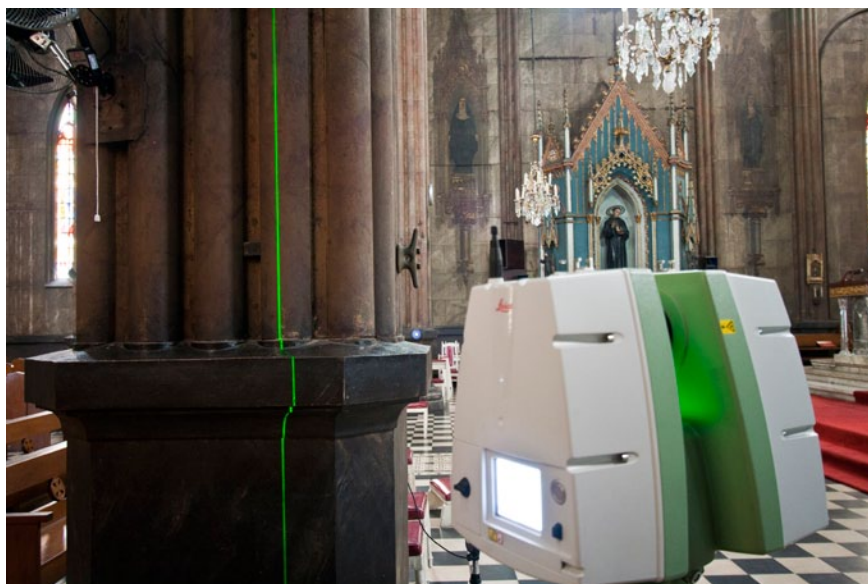
Fig. 2: Leica C10 scanning the interior of San Sebastian Basilica.
